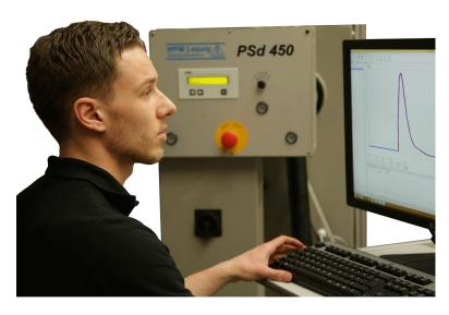
ImpaSax is the best tool to acquire measurement values and to generate reports and statistics for instrumented and not instrumented impact tests. Beside the graphic display of measurement values, automatic algorithms are included to evaluate the measured values according to ISO 14556.
